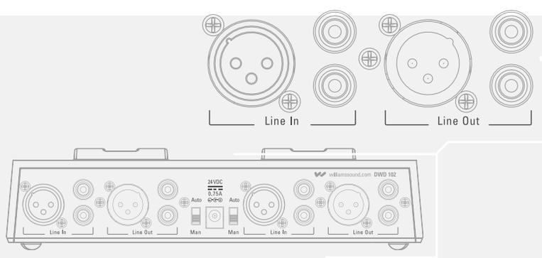
**Example 1.** Place a DLT 300 transceiver into the Dock, and easily bring audio from an outside source to listeners within a Digi-Wave system. When the input is connected to an audio source (sound system, media player and so on), the Dock allows the Digi-Wave transceiver to function much like a base station, transmitting audio to portable units.
