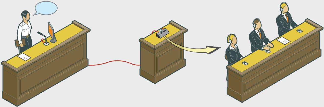
**Example 2.** You can also use the Digi-Wave Dock to deliver audio created within a Digi-Wave system to listeners of a separate sound system. Place a DLT 300 transceiver or DLR 360 receiver into the Dock. When the output is connected to a sound system or powered speaker, the Dock allows the transceiver/receiver to function like a base station receiver that connects a portable system to a fixed system.
